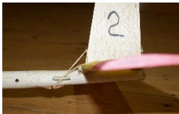
**Left:** pylon, as mentioned. (Spencer’s is single thickness.) **Right:** the d/t line must not become caught under bands.
