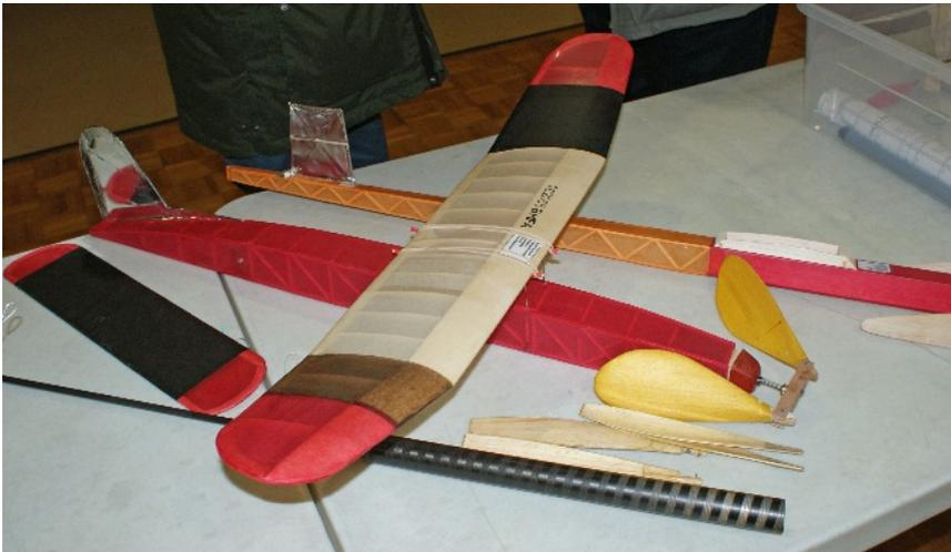
*Martin McHugh displays a new Coupe fuselage (background), a Bazooka (AM 2/1950) in the centre (well named, as I remember from seeing designer Norman Marcus launching one.) In foreground is fibreglass tube Coupe fuselage: from fishing rods, of course.*
